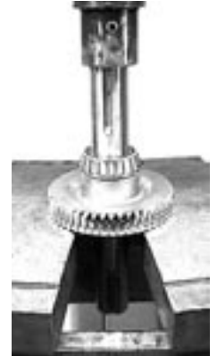
FIGURE 5 – Removal of Worm Gear and Bearing Cone
