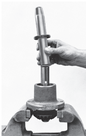
FIGURE 10 – Oil Seal Installation
