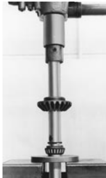
FIGURE 7 – Reassembly of Gear and Bearing Cone
