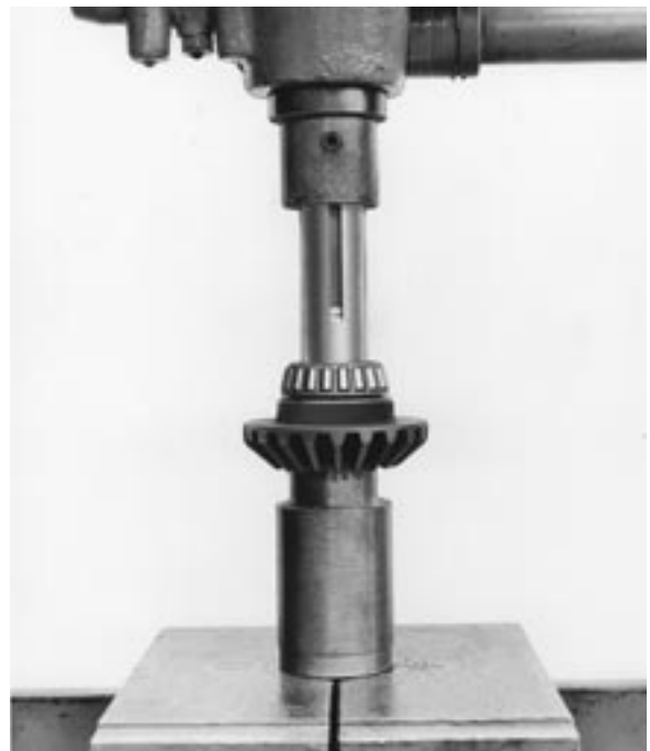
FIGURE 5 – Pressing Shaft out of Bearing and Gear
